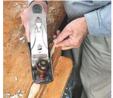
▲ Pic. 7 Using the V-cradle and a smoothing plane to create a decorative flat
